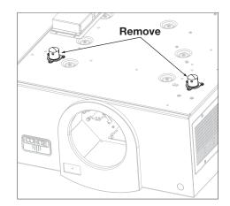
**Install Ceiling Mount Adapters/Projector Stands:** For ceiling installations, the adapters bring the attachment points for the projector mounting rails (included with the projector ceiling mount kit) from the bottom of the projector up and around the AutoScope lens motor housing. For floor installations (where the projector is upright), the adapters allow the projector to lie flat on the mounting surface.
